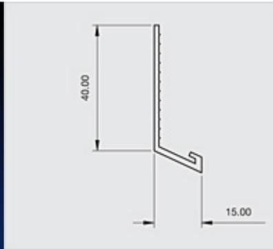
Locally manufactured from recycled plastic, Renderplas PVC bellcast beads / drip beads are designed for function and speed on all external rendering applications. Discreet but strong, all beading gives a perfect finish to through colour render and is equally suitable for sand and cement
