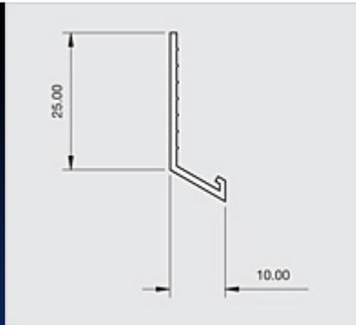
Locally manufactured from recycled plastic, Renderplas PVC stop beads are designed for function and speed on all external and internal rendering and plastering applications. This lightweight profile is designed for external wall insulation and timber frame with thinner renders and where backgrounds are even
