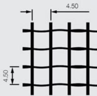
Woven from glass fibres coated in a special latex that is resistant to chemicals and alkalines Rendermesh adds strength, prevents cracks at areas of stress and protects against impact damage such as that can occur when ladders are leant against a wall. Rendermesh is suitable for use in all render, EWI, ETICS and plaster applications
