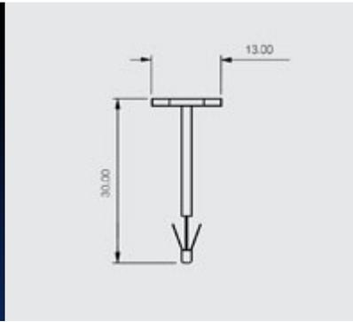
Renderplas plastic fixing pins for insulation board offer a fast simple way to install mesh beads on insulation panels. The carefully engineered tree design provides maximum grip and an exceptionally small piercing point making them very easy to use
