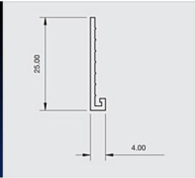
Locally manufactured from recycled plastic, Renderplas PVCu small wing stop beads are designed for economy and speed on external and internal rendering and plastering applications where the substrate is even
