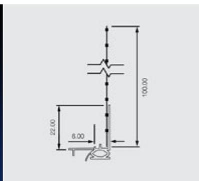
Renderplas PVC super thermal reveal beads with integrated thermal gasket to enhance insulation and protect reveal render from buffeting and continual window and door activity. Designed to protect frames and surfaces in reveals super thermal reveal beads are made with 100mm of glass fibre reinforcement mesh to extend the life of render and EWI systems
