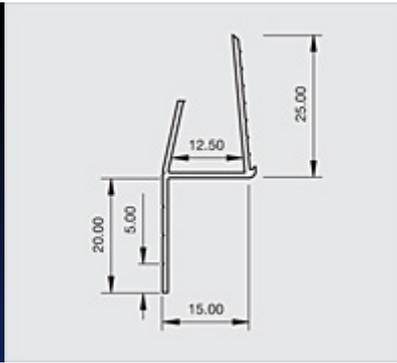
Locally manufactured from recycled plastic, Renderplas PVCu architrave shadow gap beads are designed for plasterboard to quickly and accurately form a shadow gap and provide a superior clean finish. Used at the edges of the plasterboard next to door frames, ceilings and skirting boards where the adjacent finish is designed to be seen
