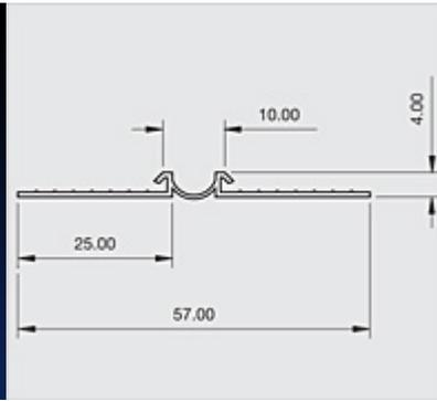
Locally manufactured from recycled plastic, Renderplas PVC movement joint / expansion joint beads are designed for areas of render over 20 square metres and should be specified every 4-6 metres, over structural movement joints and changes of background giving a discreet attractive finish. Also for use as an internal corner with plasterboard
