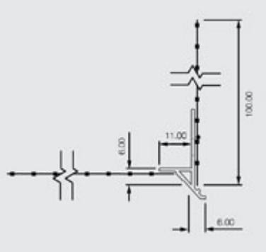
Renderplas PVC reveal head beads with drip detail and glass fibre reinforcement mesh. Designed for function and speed of installation at the head of all EWI and thin coat rendered reveals
